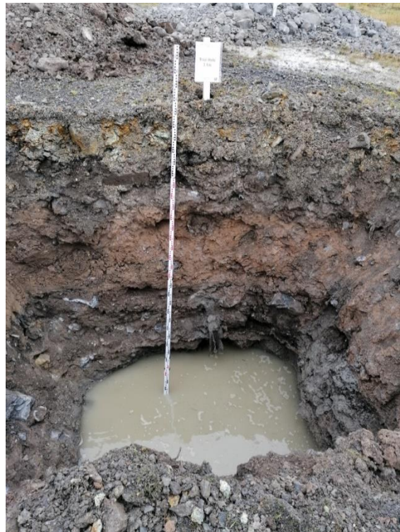
Figure 18: Illustrates trial hole 3 & shows the different horizons within the trial hole.
