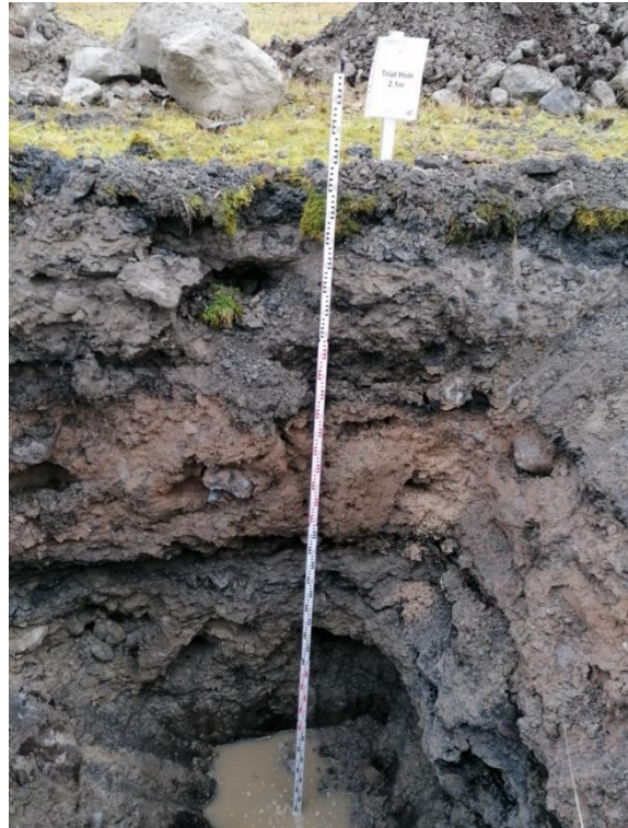
Figure 12: Illustrates trial hole 1 & shows the different horizons within the trial hole.
