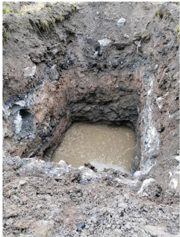
Figure 6: Illustrates trial hole 1 & shows the different horizons within the trial hole.
