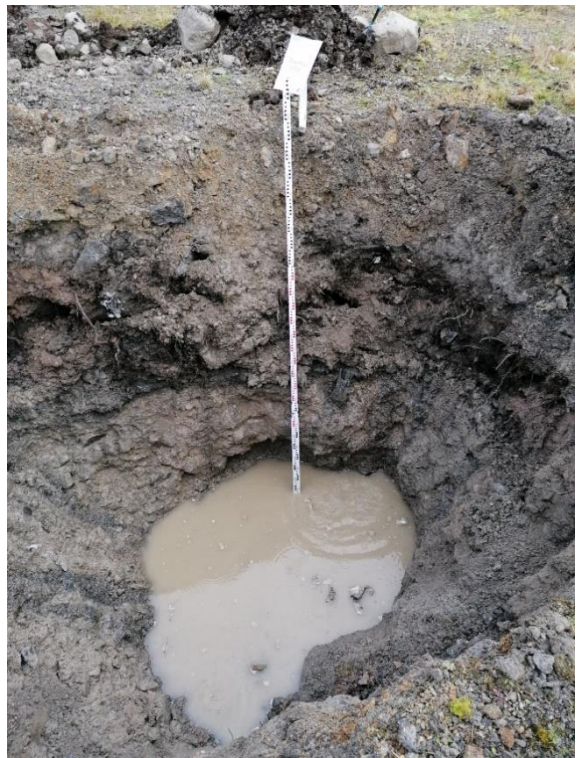
Figure 30: Illustrates trial hole 5 & shows the different horizons within the trial hole.
