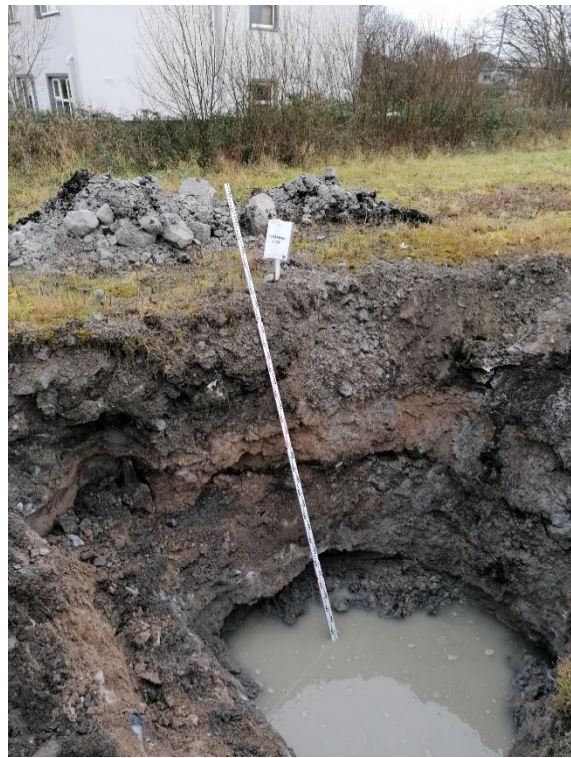
Figure 24: Illustrates trial hole 4 & shows the different horizons within the trial hole.
